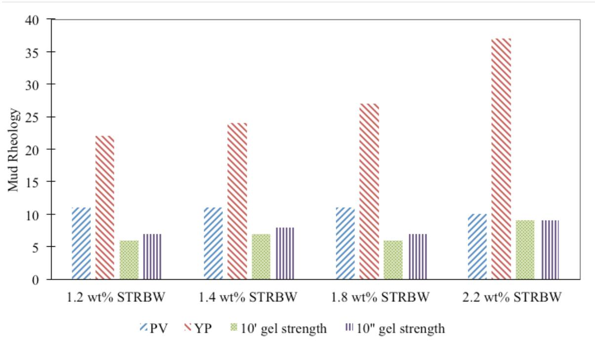
**Figure 7** Effect of different concentrations of STRBW on rheology
