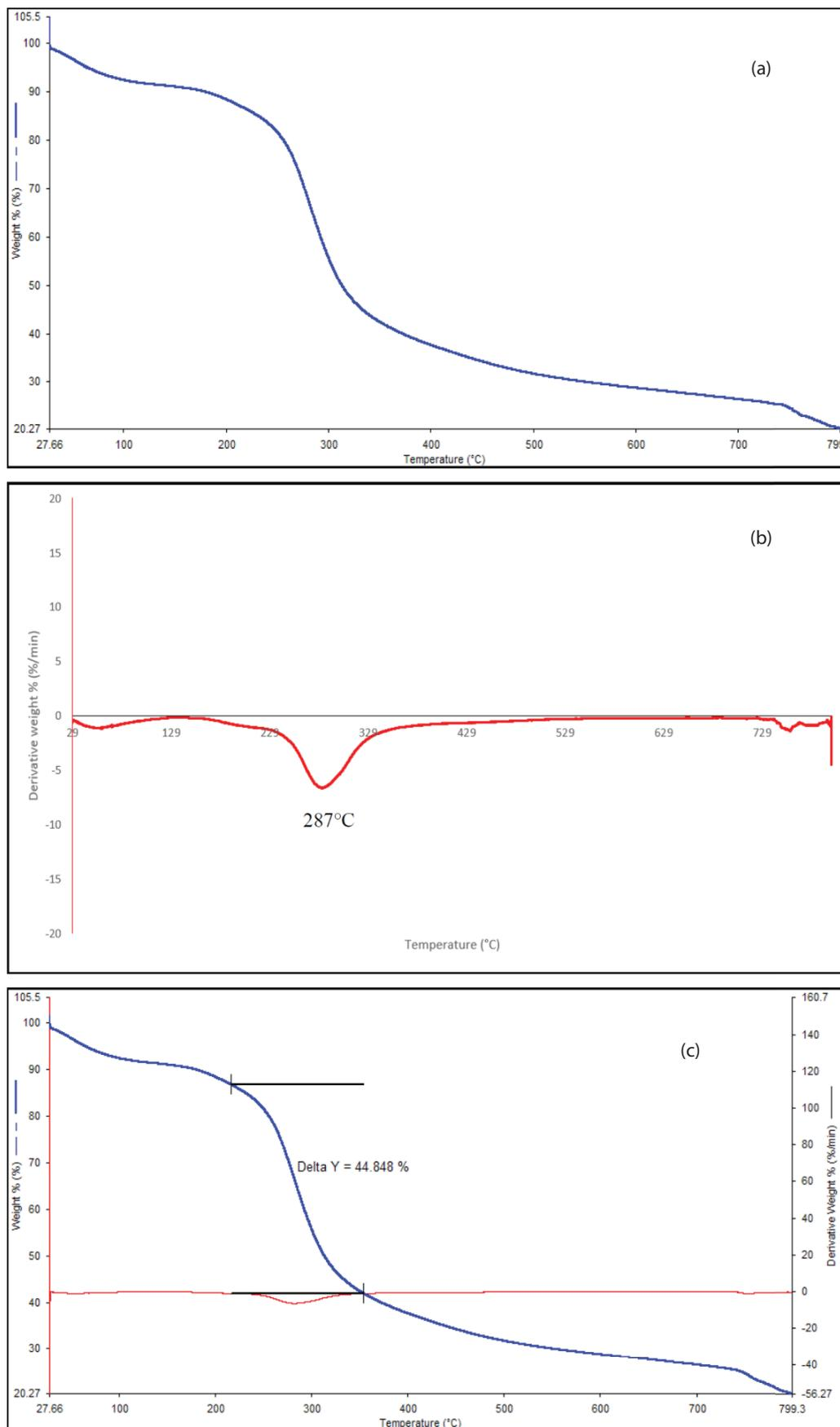
**Figure 1** Thermal stability analysis of STRPB using TGA. a) Thermogravimetry, b) Derivation Thermogravimetry and c) DTG Curves
