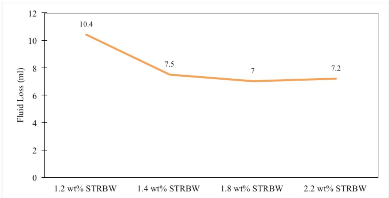
**Figure 8** Effect of STRBW with different concentration on fluid loss
