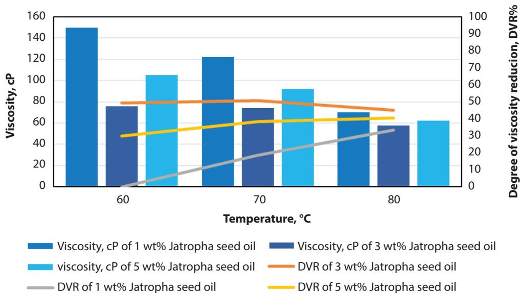
Figure 3 Viscosity and DVR % for all concentrations and temperatures
