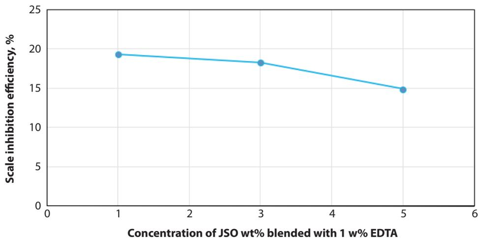
**Figure 5** Scale inhibition efficiency chart
