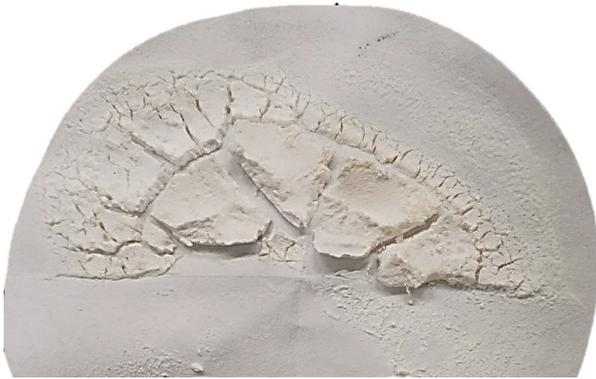
**Figure 4** Barium sulfate scale
