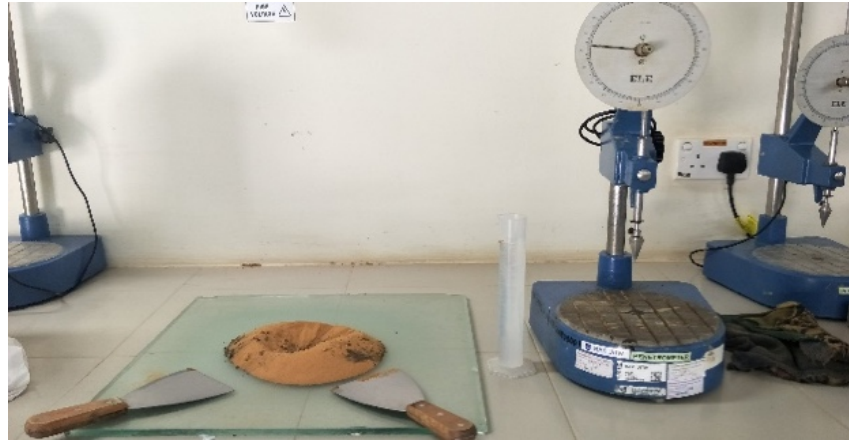
Figure 4. The preparation of soil-geopolymer mixture on liquid limit test
