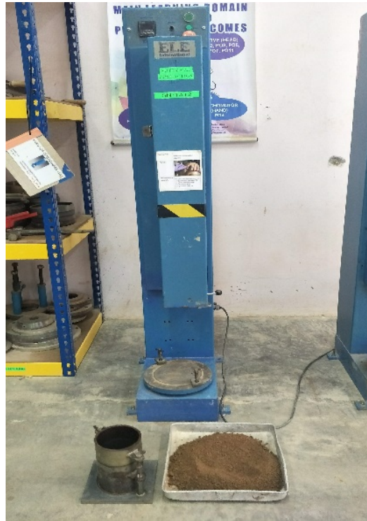
Figure 8. The compaction test using Standard Proctor test
