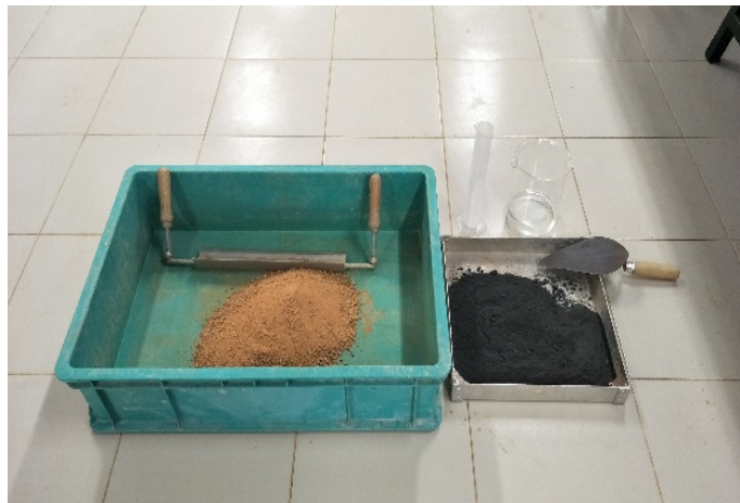
Figure 7. The preparation of soil-geopolymer mixture for compaction test
