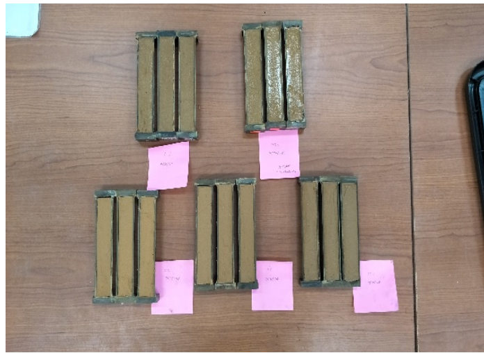
Figure 6. The Shrinkage test of soil-geopolymer mixture
