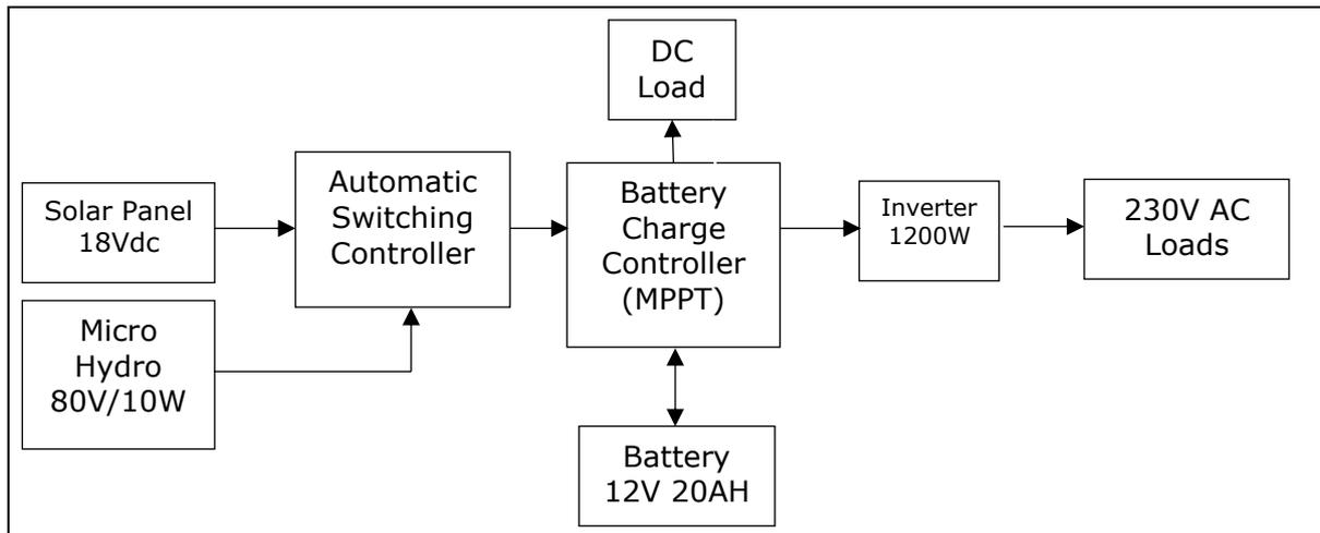
Figure 1. Block diagram of Micro Solar-Hydro Power Generation System
