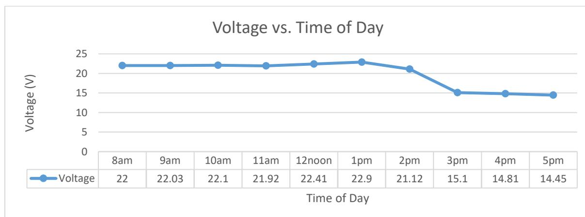
Figure 3 Open-circuit Voltage Test versus Day Time
