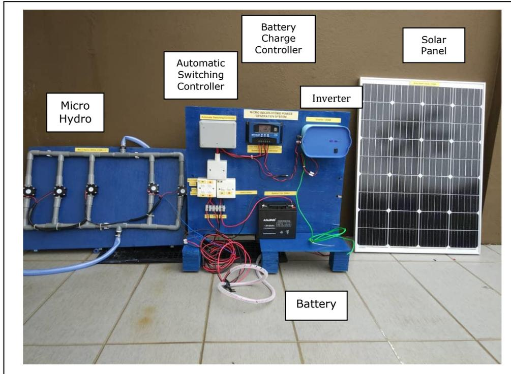
Figure 2 The Prototype of Micro Solar-Hydro Power Generation System
