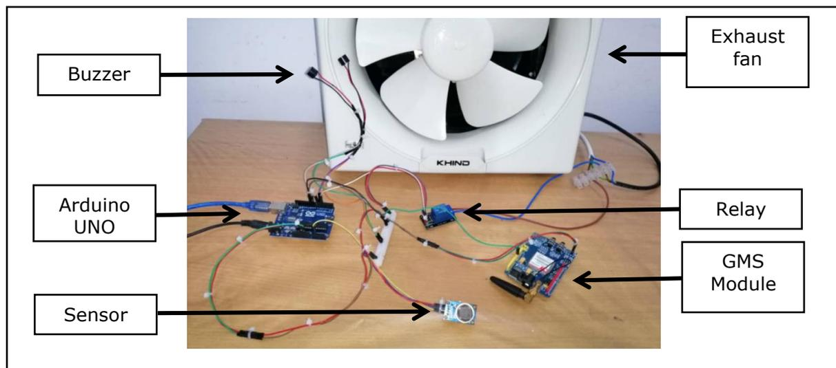
Figure 3: Prototype of Smart Gas Detection System
