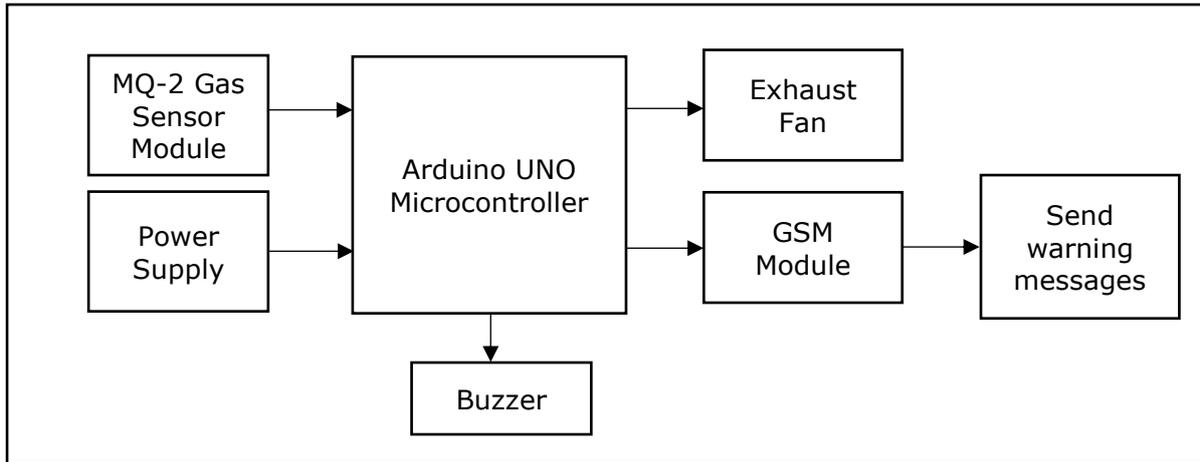
Figure 1: Gas Detection System Block Diagram
