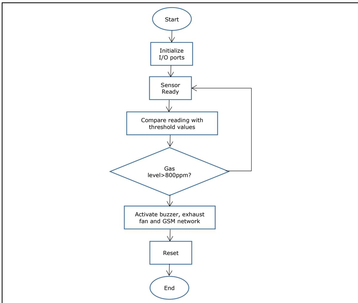
Figure 2. Flow Chart of the Gas Detection System
