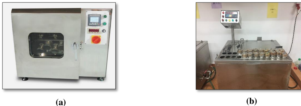
Figure 2. (a) Lab IR Dyeing Machine and (b) Water Bath Exhaustion Dyeing Machine.
