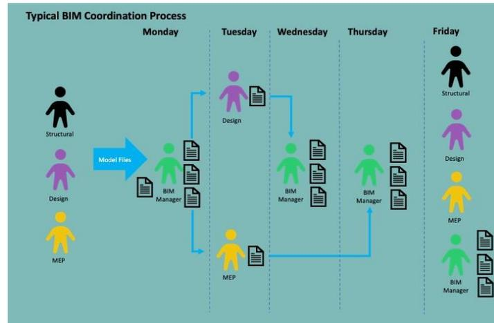
**Figure 1: Typical BIM Coordination Process (Applied Software Technology, 2016)**
