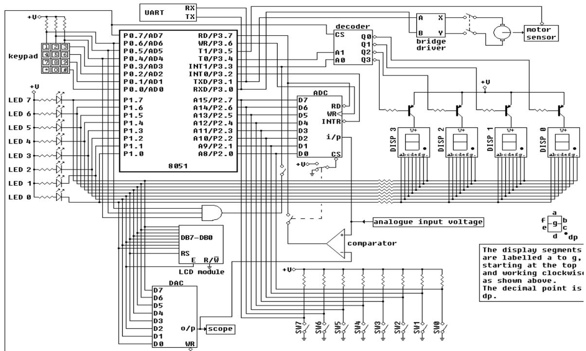
Figure 3: Logic diagram of EdSim 51 simulator.
