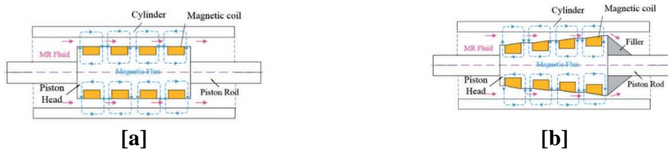
Figure 6: Schematic diagrams of MR damper with electromagnetic coils [a] Typical multi coils damper [b] Proposed multi coils MR damper design (Zheng et al., 2016).
