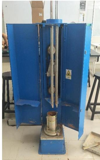
Figure 8: Standard Proctor test
