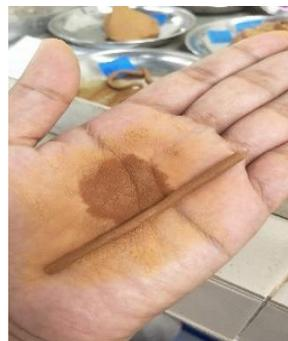
**Figure 5: Plastic Limit test**
