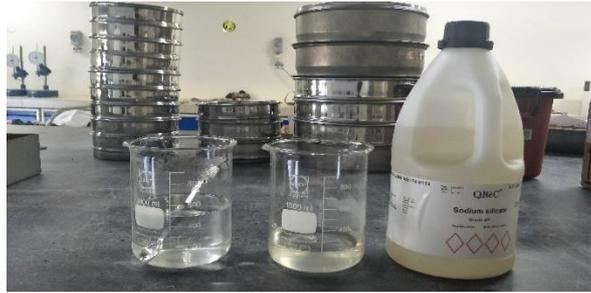
**Figure 1: Alkaline Solution Preparation**
