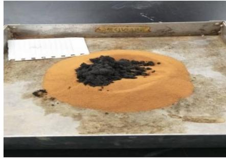
**Figure 3: Laterite mix with geopolymer mixed before experimental tests conduct.**
