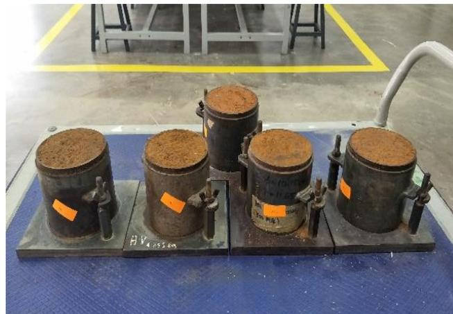
Figure 9: Compaction sample of various percentage of soil-geopolymer
