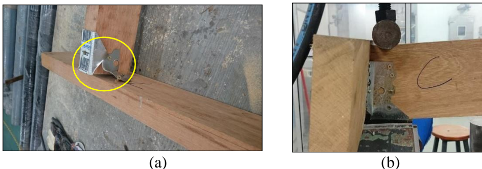
Figure 9: (a) Failure on joist hanger for sample SST1 (b) Failure on joist hanger for sample SST2
