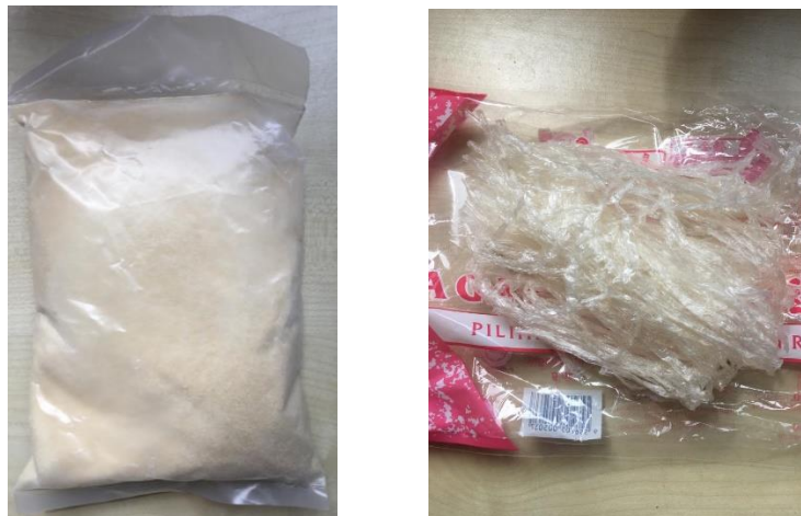
Figure 1: Gelatin powder (left) and agar strips (right) used as phantom base in this experiment
