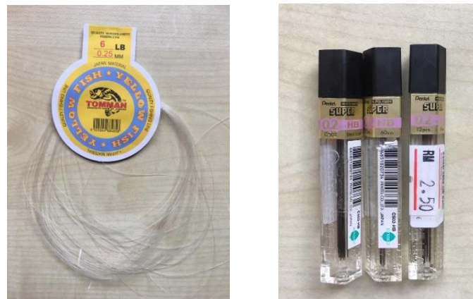
Figure 3: Nylon (left) and pencil lead (right) used as filaments in this experiment
