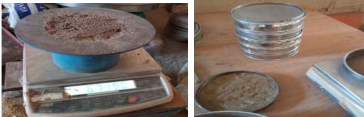
Figure 2: (a) Cylinder for measuring bulk density; and (b) a nest of sieves for sieve analysis
