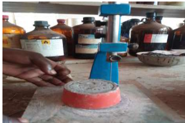
Figure 4: (a) Schematic diagram of a vicat apparatus; b) Performing initial and final setting time with Vicat apparatus
