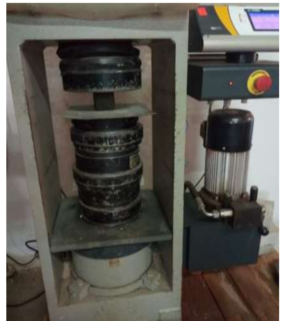
Figure 5: a) Schematic diagram; b) Compressive strength test with mortar cube being crushed
