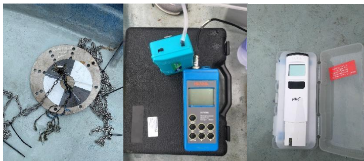
Figure 2: Apparatus and instruments used for data collection (from left Secchi disk, DO meter, and pH meter equipped with temperature detector)
