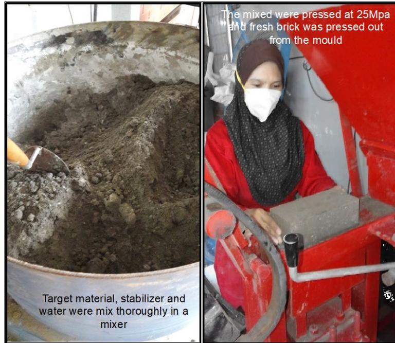
**Figure 2.** Fabrication of LSP Bricks Materials were thoroughly mixed and pressed.
