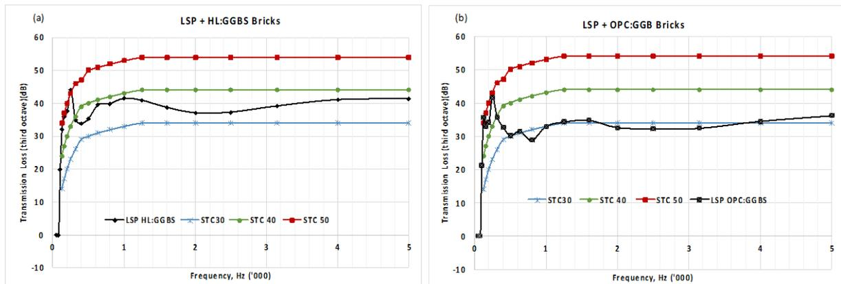
**Figure 4:** Transmission loss vs frequencies for LSP Brick stabilised with (a) HL:GGBS and (b) PC:GGBS
