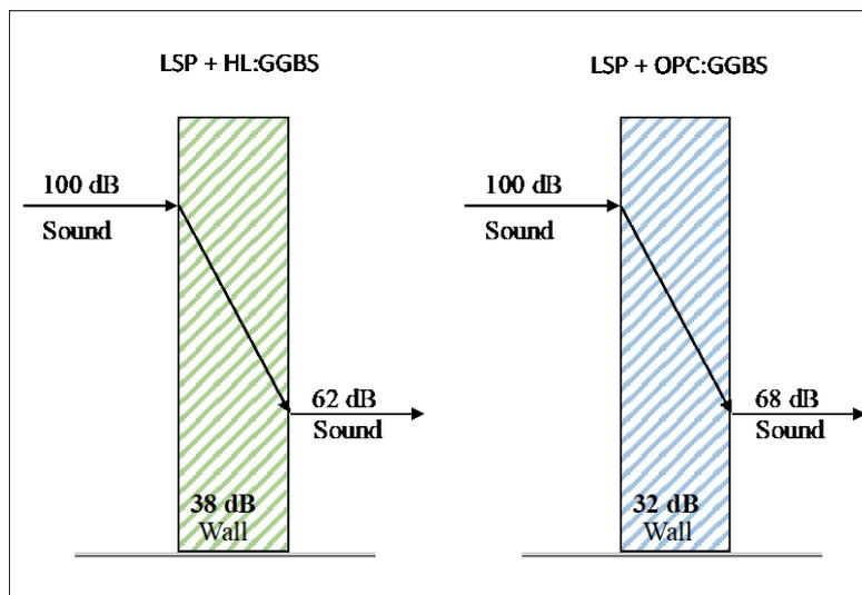
**Figure 5:** Schematic drawing of sound transmission loss of LSP Brick-wall
