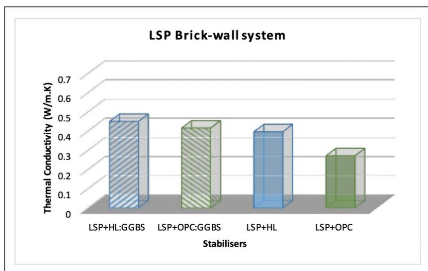
Figure 6: Thermal conductivity vs stabilisers of LSP Bricks
