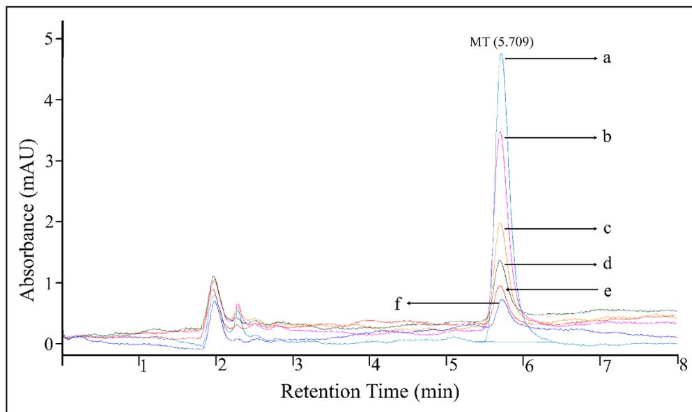
Figure 4: Standard curve chromatograms of Methyltestosterone; (a) 600 µg/L, (b) 400 µg/L, (c) 200 µg/L, (d) 100 µg/L, (e) 50 µg/L and (f) 25 µg/L.
