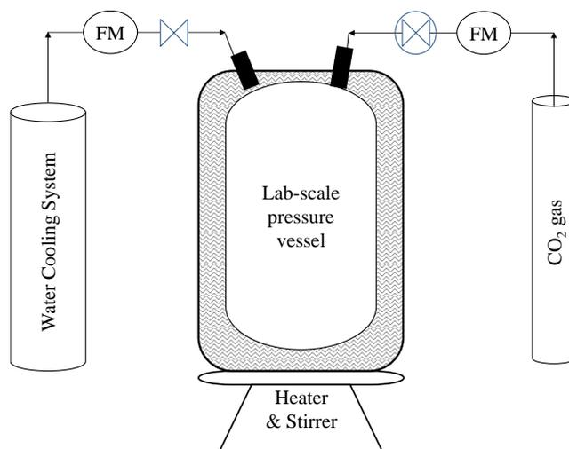
**Figure 2: Schematic diagram of experimental; set-up of high-pressure autoclave (Amar model P2313)**
