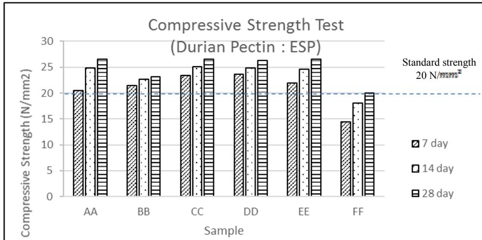
**Figure 4:** Result of compressive strength test (ratio of durian pectin: ESP)
