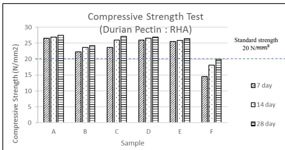
**Figure 3:** Result of compressive strength test (ratio of durian pectin: RHA)
