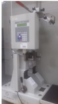
**Figure 5:** Charpy test machine
