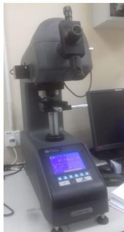
**Figure 6:** Vickers hardness test machine
