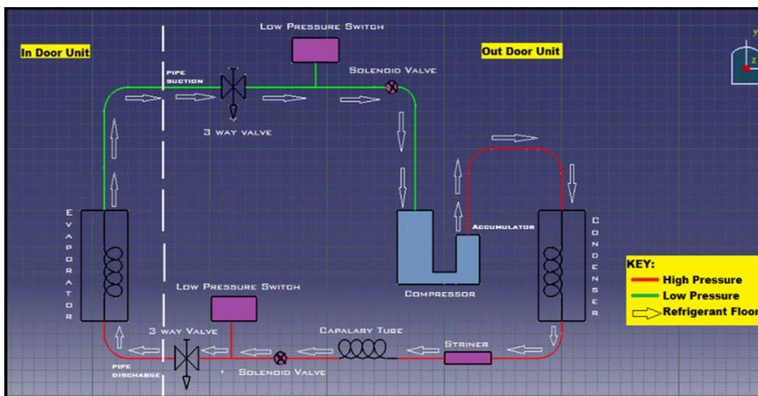
**Figure 2:** Schematic drawing of modified outdoor unit
