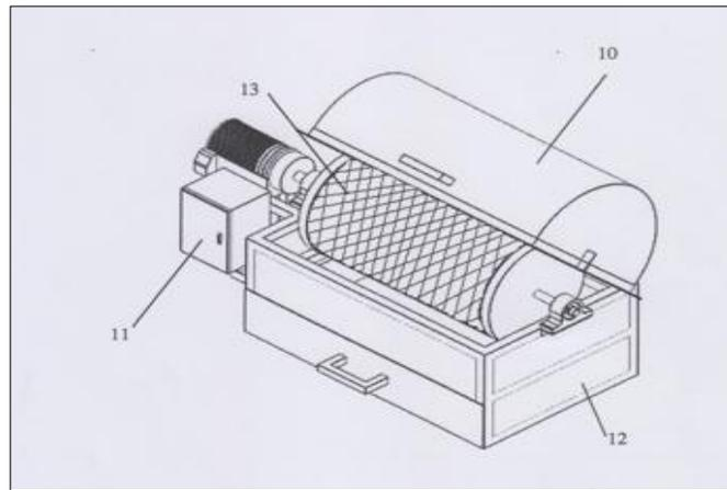
**Figure 8:** Shallot Peeling Machine Design
