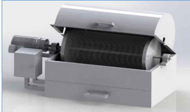
**Figure 9:** Shallot Peeling Machine 3D Design
