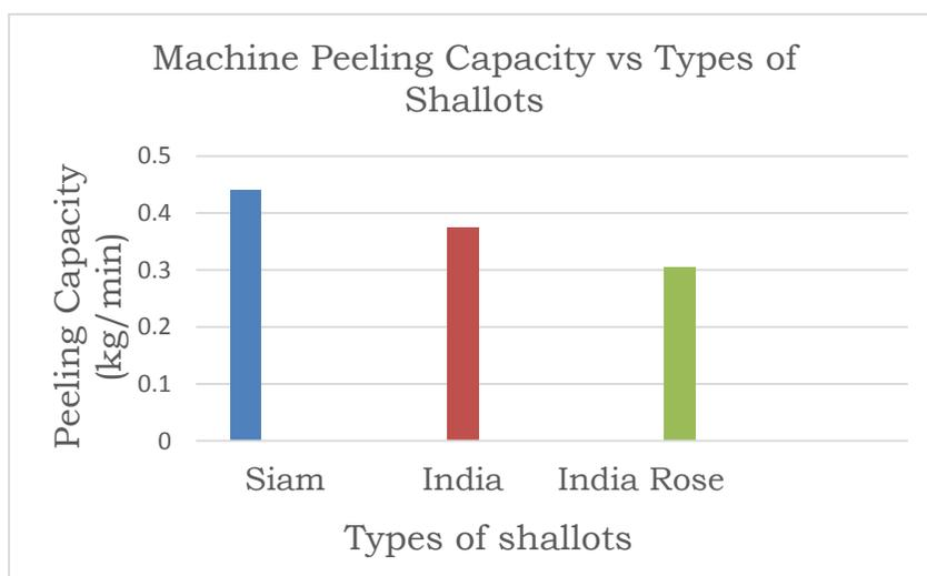
**Figure 13:** Machine Peeling Capacity for Three Different Shallots
