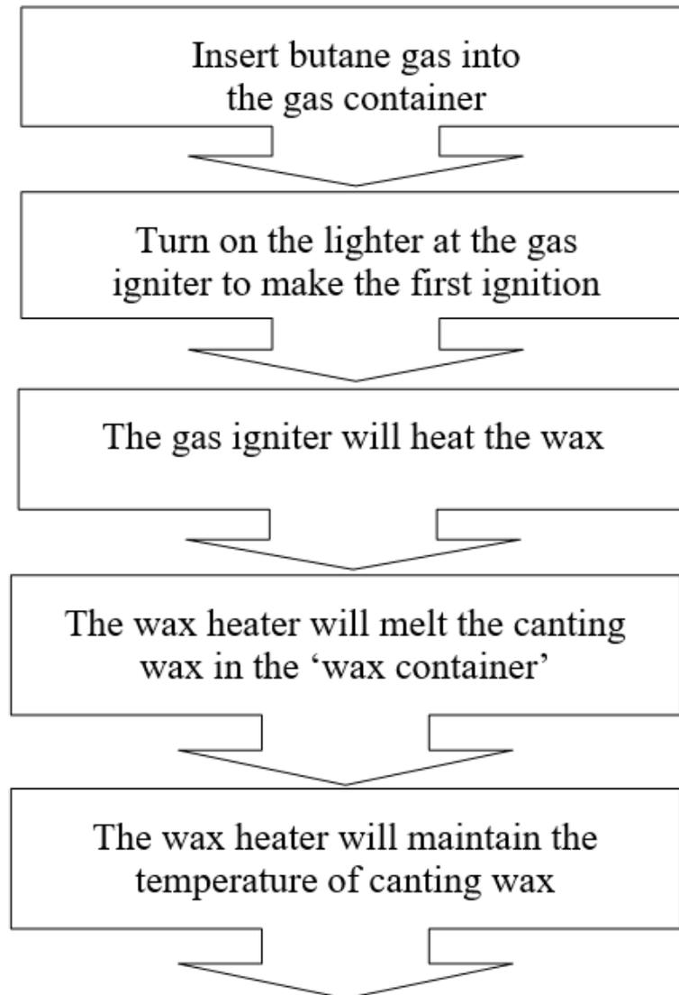
**Figure 2:** Process flow of gas *canting* tool
