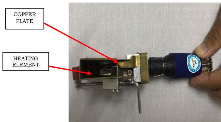
**Figure 4:** Copper plate at the aluminium soldering iron holder
