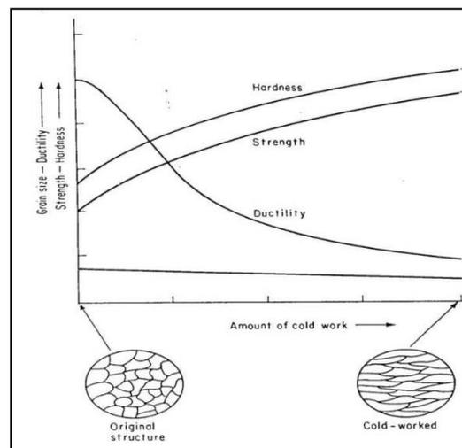
**Figure 3:** Effect of cold working on tensile strength, hardness, ductility and grain size (the curve below ductility represents the change
