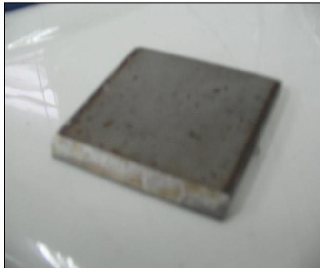
**Figure 4:** Stainless Steel 316L (sheet)
