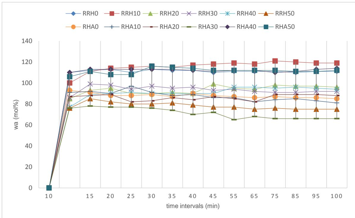
**Figure 3:** Water absorption value for RRH-RHA-concrete after 28 days of water cured
