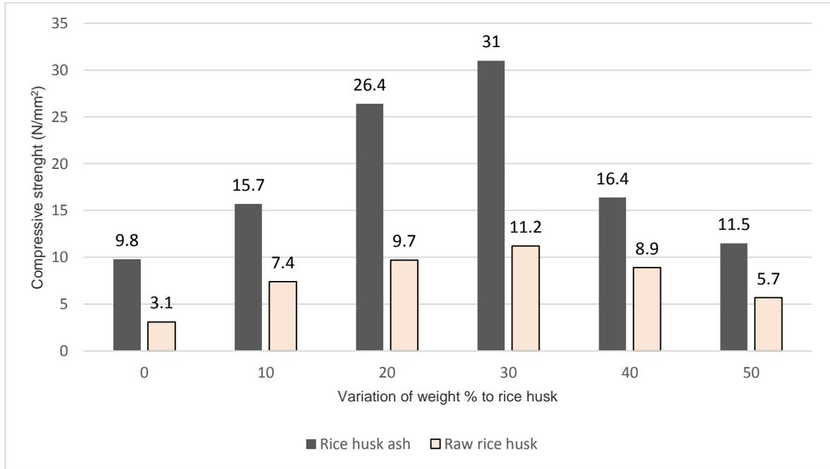
**Figure 2:** Variation of 28 days compressive strength for different mixture proportion
